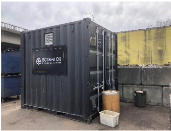
Example of 10 ft seacan 8'(w) x 10'(l) x 8' 6" (h) steel shell with 660 liters secondary spill containment
